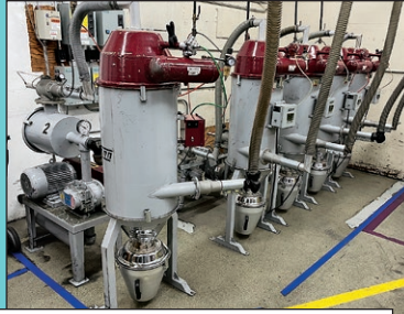
Wittman DryMax E1200 Central Dryer System with (16) Hoppers and (5) Pumps (New 2013)
