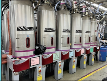
Wittman DryMax E1200 Central Dryer System with (16) Hoppers and (5) Pumps (New 2013)
